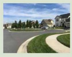
2. This loop lane reduces the need for backing up of vehicles and creates about 10% less impervious cover than Option 1.
